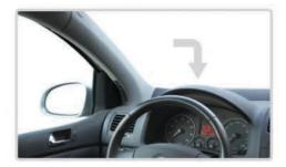
Base of windshield, no metallic obstructions (windshield wipers, wires, etc.).
